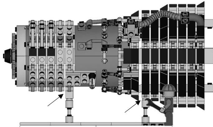
A stronger support has been designed, built, and tested on the particular customer's unit. And it has significantly improve the sturdiness of the engine support.
